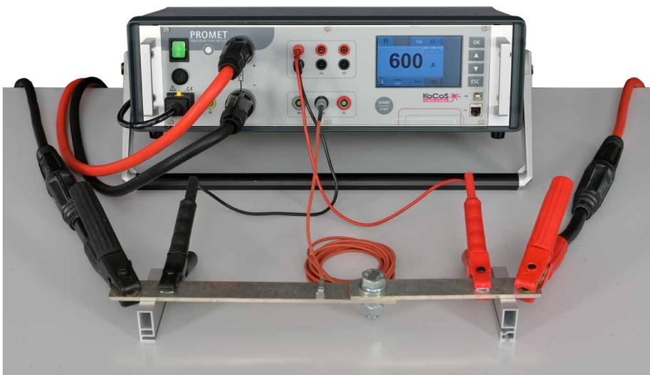
Fig. 2: Measurement setup with PROMET R600 micro-ohmmeter
