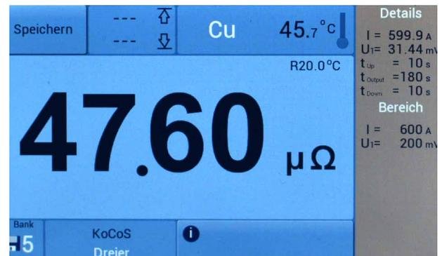
Fig. 5: Measurement result with uncompensated value and value compensated to 20 °C
