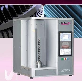
Shape and position tolerances in accordance with ISO 1101 for the entire test object, freely definable sections or individual areas can be measured:
